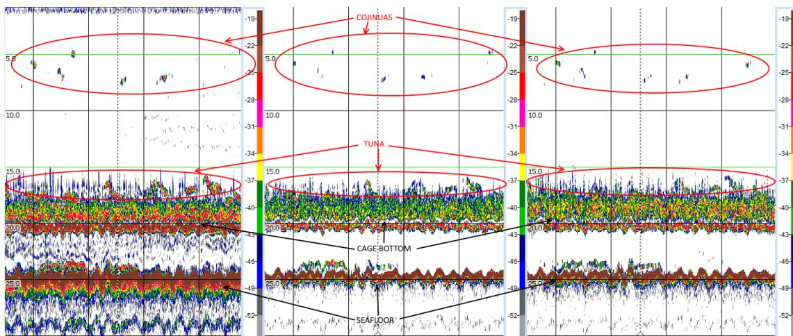
Figure 4. Example of TS echogram showing cojinúas and tunas at the three frequencies 38 (left), 120 (middle) and 200 (right) kHz. The minimum threshold is set at -55 dB.
