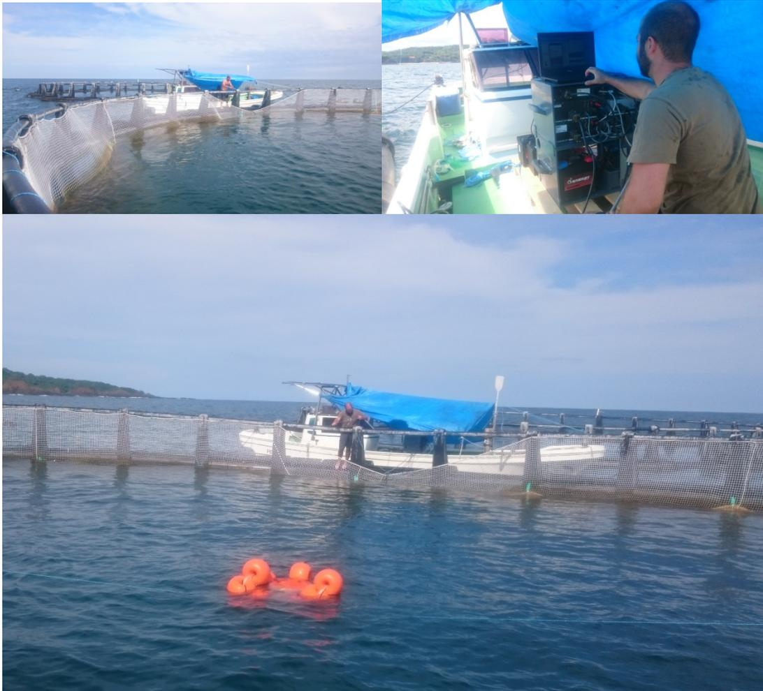
Figure 2. The offshore cage that contained the tuna. Attached to the cage, the fishing boat “Kihada Maru”, where the acoustic equipment was installed, and the transducers in the middle of the cage.
