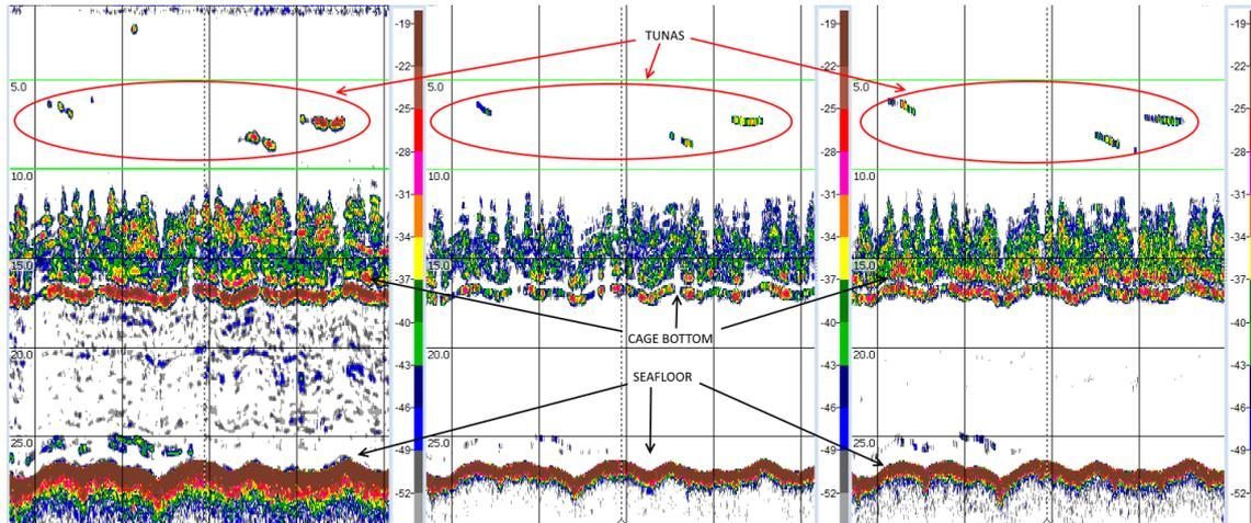
Figure 3. Example of TS echogram showing tunas at the three frequencies 38 (left), 120 (middle) and 200 (right) kHz. The minimum threshold is set at -55 dB.
