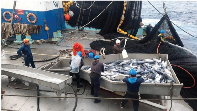
**FIGURE 1.** (a) Double-mesh brailer filled with fish; and, (b) a hopper on the main deck of a vessel.
