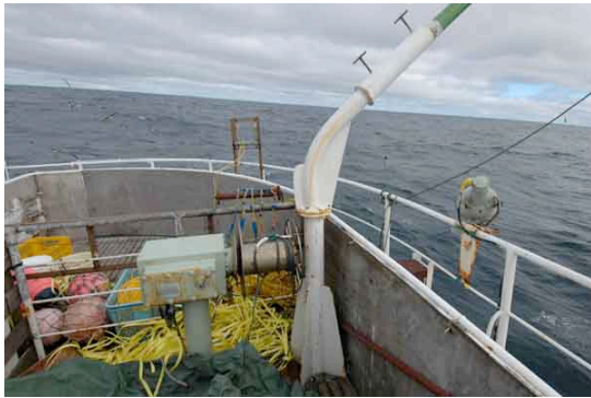
Figure 6. Port tori pole davit and winch.
