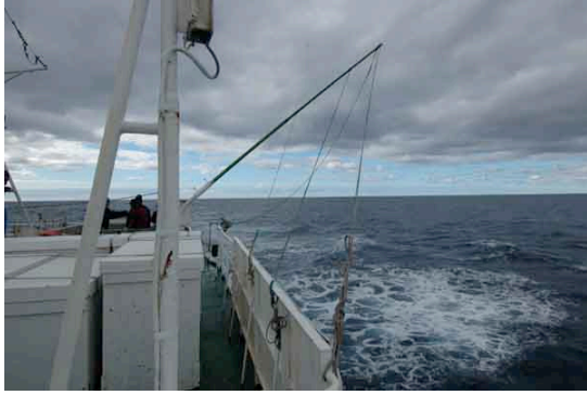
Figure 7. Port tori pole
