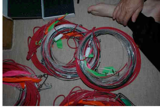
Figure 14. Star-Oddi TDRs taped to branchlines at the hook.
