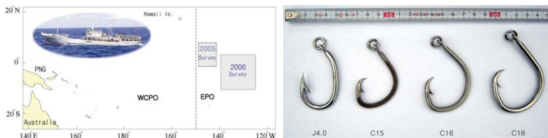
Figure 2-1. Fishing gear for circle hook experiment. One type (J-4) of traditional tuna hook and three types (C15, C16, C18) of
