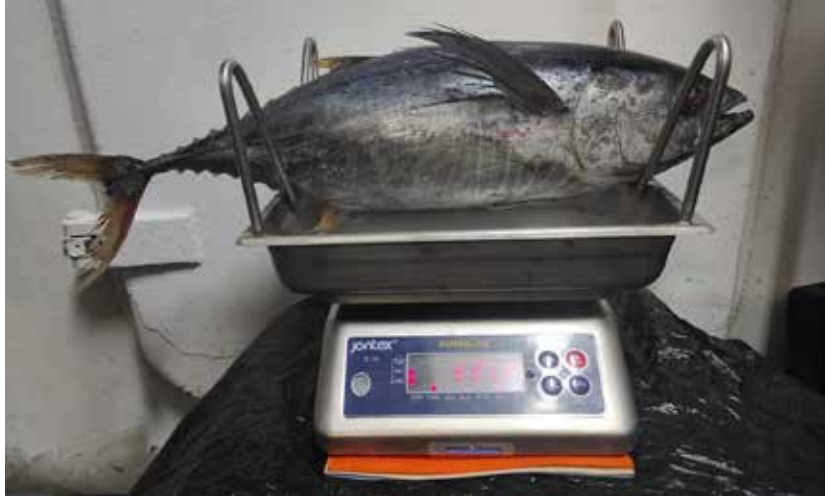
FIGURE 4. Portable scale with custom tray and anti-vibration base. FIGURA 4. Balanza portátil con bandeja modificada y base antivibraciones.
