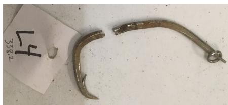
Breaking (unbending/opening) strength influenced by soak time, metal type, hook size and forging:
