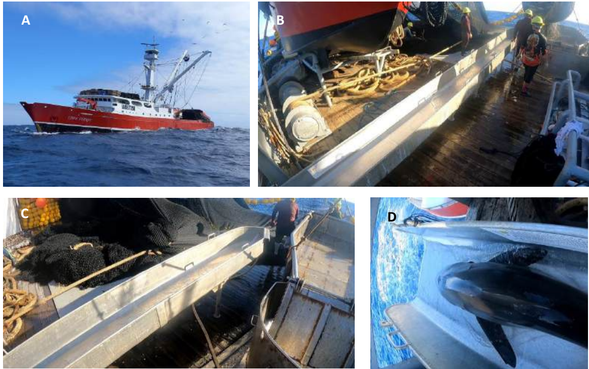
Figure 1.- (A) Cape Ferrat (Cape Fisheries) purse seine; (B) Cape Ferrat's hopper and bycatch release ramp; (C) First section of the release ramp with a connected water hose and showing the 0.45-meter gap between the hopper and the ramp that allows a crew member to be positioned in this space to assist with bycatch release; (D).
