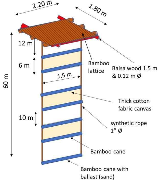
**FIGURE 12.** Additions and modifications to improve durability of Prototype 3. Note that synthetic rope will only be used in the last batch of deployments (still pending). Deployments of 3<sup>rd</sup> quarter of 2021 consisted of NEDs with a biodegradable cotton-based rope that was successfully used and implemented in other ocean regions by some vessels of the same fleet.
