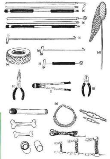
Figure 26. Equipment used to handle and release sea turtles. The United States National Marine Fisheries Service requires this equipment to be carried on board United States Atlantic longline vessels (after U.S. National Marine Fisheries Service, 2004).
