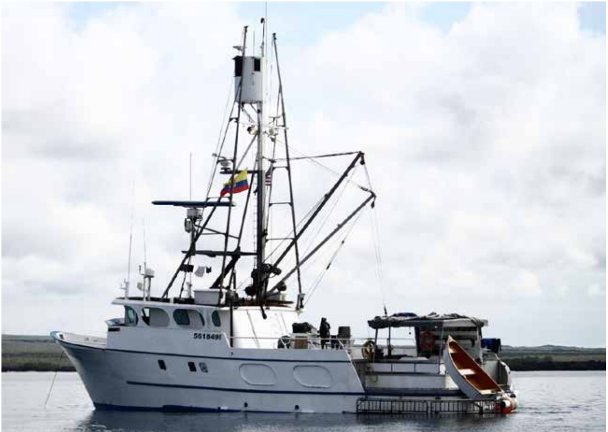
FIGURE 1. F/V Her Grace at anchor while catching bait in the Galapagos Islands National Park, Ecuador. The racks, where the fisherman stand while fishing with pole-and-line, are visible along the stern of the vessel.
