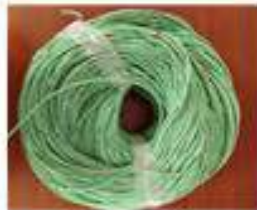
Polyethylene & polyamide mother line, 6 mm Ø
