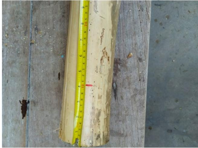
3. Drill a whole of 40mm through the bamboo cane on both sides (to insert the small bamboo canes)
