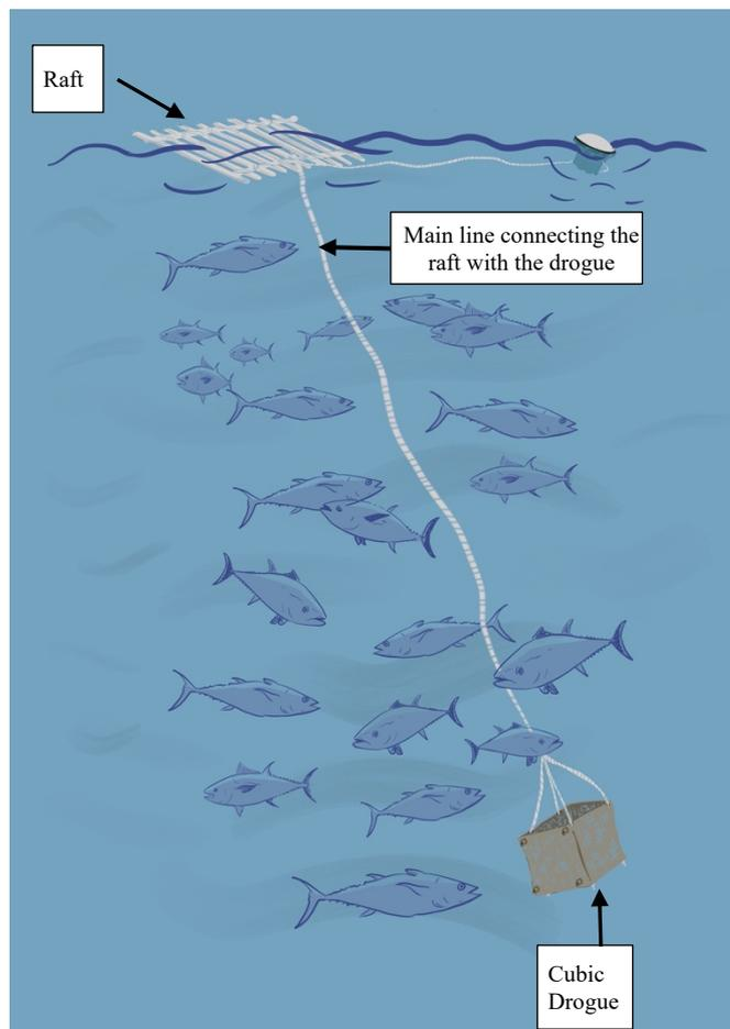
Figure 5. Conceptual drawing of the new DFAD design
