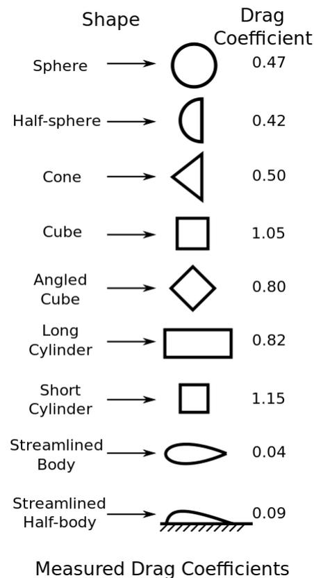
Figure 2. Measured drag coefficients for different shapes
